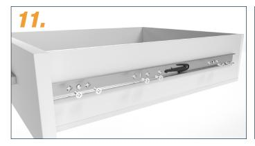
Fasten the inner rail with countersunk screws. For metal body e.g. with countersunk head screw M5x16, for wooden body, e.g. with countersunk screw 4.5x16 (available in our online shop).
