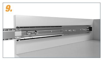
Fasten outer rail with countersunk screws. For metal body, e.g. with countersunk head screw M5x16, for wooden body e.g. countersunk screw 4.5x16 (available in our online shop).
