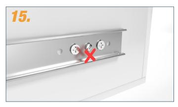
No screw heads should protrude from the rear holes.
