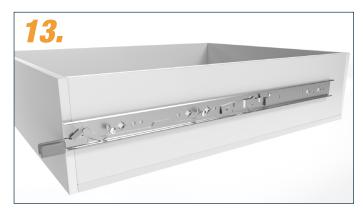
The inner rail can be fixed with screws in the slotted holes e.g. with a 4 mm round-head screw (not supplied). Screws can be optionally removed again after installation.
