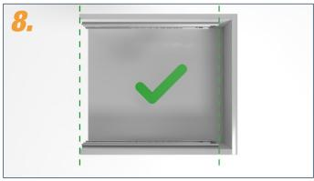
Outer rails must be flush and parallel at the front.
