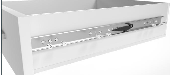
Fasten the inner rail with countersunk screws. For metal body e.g. with countersunk head screw M5x16, for wooden body, e.g. with countersunk screw 4.5x16 (available in our online shop).
