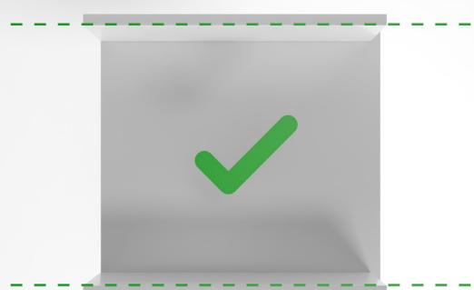
Side walls of the cabinet body must be parallel.
