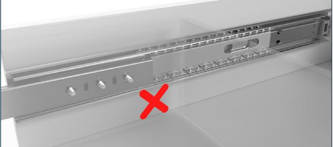
Incorrect handling can cause the rail to tilt. No liability is accepted for damage to the ball cage caused by incorrect reinsertion.
