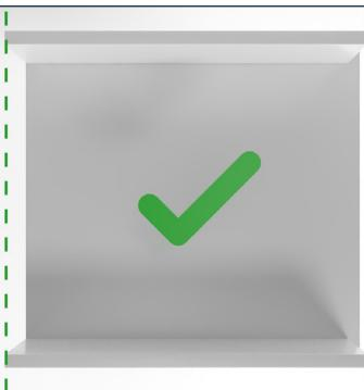
Side walls of the cabinet body must be flush at the front.
