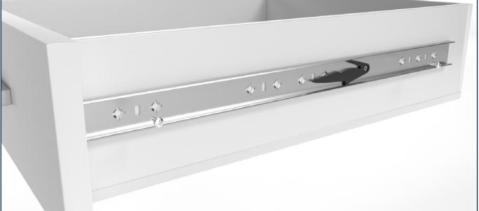
The inner rail can be fixed with screws in the slotted holes e.g. with a 4 mm round-head screw (not supplied). Screws can be optionally removed again after installation.
