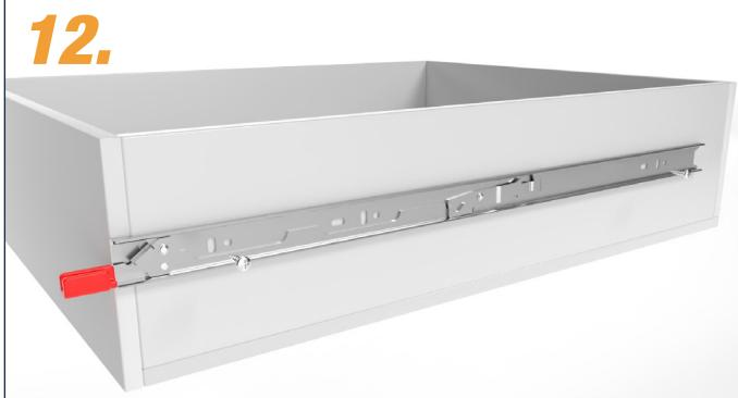
The inner rail can be fixed with screws in the slotted holes e.g. with a 4 mm round-head screw (not supplied). Screws can be optionally removed again after installation.
