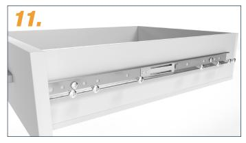
Fasten the inner rail with flat head screws. For metal body e.g. with flat head screw M6x16, for wooden body, e.g. with flat head screw 6x16 (available in our online shop).
