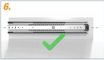
Side walls of the cabinet body must be flush at the front.
