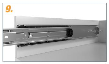
Fasten outer rail with screws. For metal body e.g. with flat head screw M6x16, for wooden body e.g. flat head screw 6x16 (available in our online shop).
