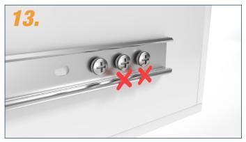
No screw heads should protrude from the rear holes.
