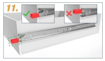
When installing the inner rail, the locking lever must point upwards.
