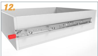
Fasten the inner rail with countersunk screws. For metal body e.g. with flat head screw M6x16, for wooden body, e.g. with flat head screw 6x16 (available in our online shop).
