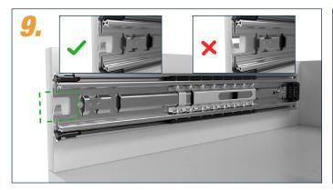
We recommend that the tab on the outer rail should point upwards.
