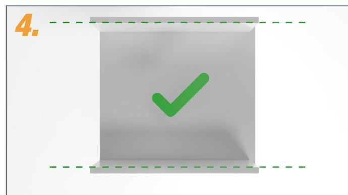
Side walls of the cabinet body must be parallel.
