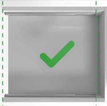
Outer rails must be flush and parallel at the front.
