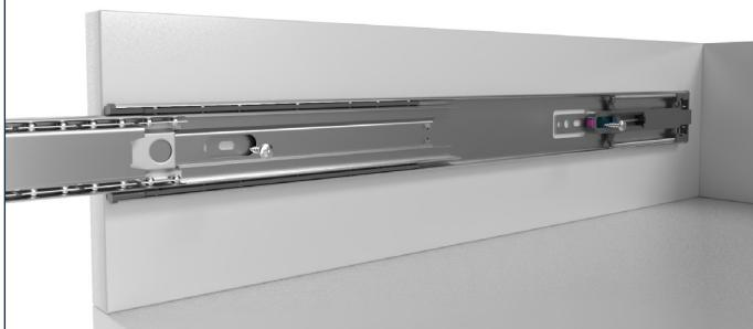
The outer rail can be fixed in the slotted holes with screws and still be aligned. e.g. with 4 mm round-head screw (not supplied).
