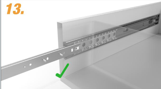
Before installation, the ball cage must be pushed forward.
