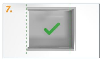
Outer rails must be flush and parallel at the front.
