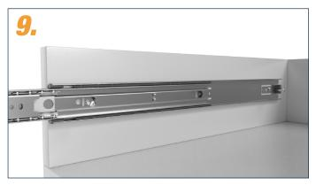
Fasten the outer rail with screws. For metal body e.g. with flat head screw M4x8, with wooden body e.g. with flat head screw 4x14 (available in our online shop).
