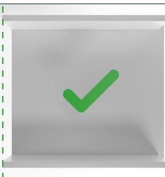
Side walls of the cabinet body must be flush at the front.
