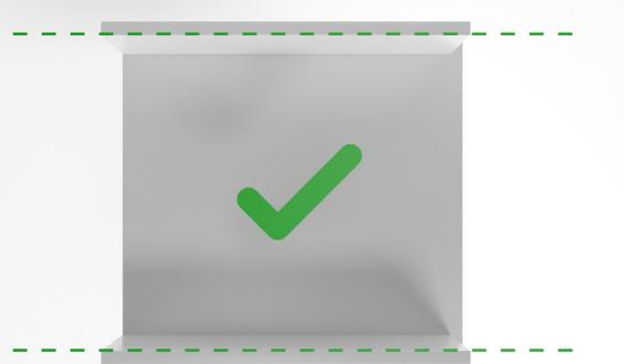
Side walls of the cabinet body must be parallel.
