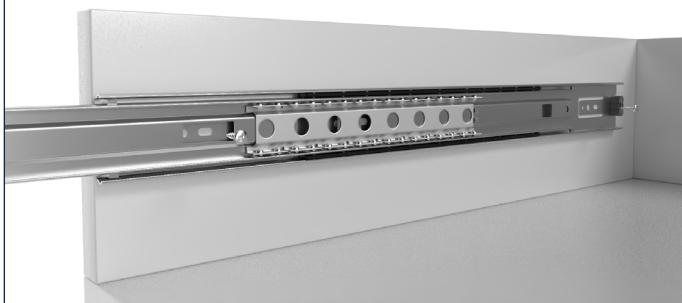
The outer rail can be fixed in the slotted holes with screws and still be aligned. e.g. with 4 mm round-head screw (not supplied).
