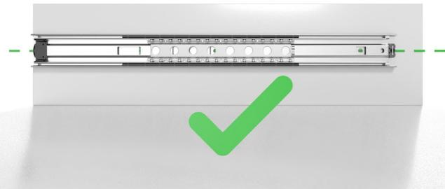
Outer rail must run parallel to the floor.
