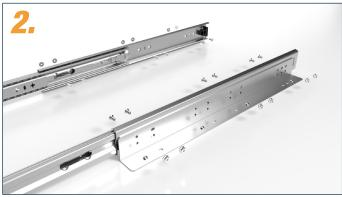
Screw heavy-duty drawer slides to mounting brackets with M5x10 countersunk screw and M5 nut with flange. (supplied)
